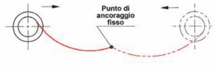
CABLE REEL ON MOBILE APPLICATION, 2 DIRECTION UNCOILING
